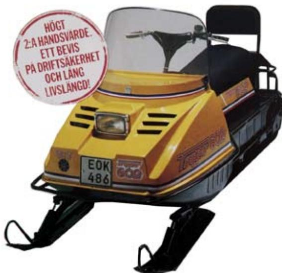
Next model Trapper 600, new model and design, 440 Rotax engine and 1+1 gear box. Was manufactured in Kurikka Velsa OY, Lynx workshop. At the time (1979) Teo Lehtimäki worked with raw-materials and had his first experience/contact with Trapper. Trapper 602 came out 1980-1981 with Rotax 503 engine and new gear box. In addition to this in 1980 the Trapper 602 was available with Rotax 444 L/C and 1981 Rotax 464 L/C engine.
